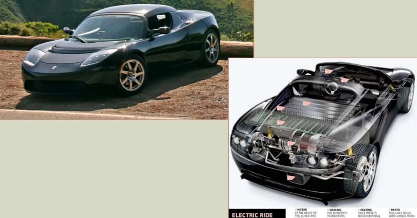
MOTOR IS A HIGH-EFRICENCY ROTOR THE BREAKTHROUGH IT'S MADE OF BRAZED COPPER. WHICH IS MORE CONDUCTIVE THAN ALLMANUM ROTOR
